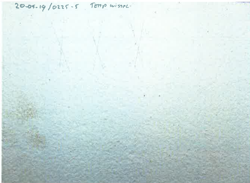
Photo 5: Adhesion after cyclic temperature test Panel 5
